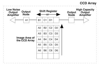
Figure 24. Array Terms for a CCD with a Dual Output Amplifier
